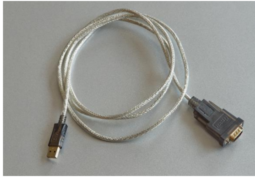
Figure 4.4 the wire for the RS232 connecting
