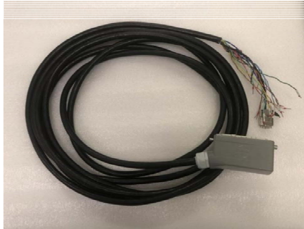
Figure 4.4 The wire for the control connecting
